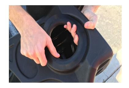
Carefully remove the MAF sensor from the stock intake box lid with a T20 Torx. Use the supplied 8-32 Screws (K), MAF Pad (J), Gasket (I) to install the sensors onto the Intake Tube (C) with a Phillips Screwdriver. Do not over tighten.
