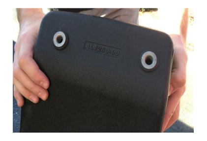
Insert the Airbox Fender Seal (T) into the Airbox (A).
