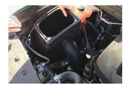
Make sure the Airbox Fender Seal (T) is sitting flat against the fender wall and not being pushed upward.
