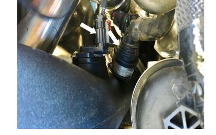
Place the Air Filter (Y) into the Airbox (A). Rotate the air filter into position as shown below and tighten the #80 Hose Clamp (Z)
