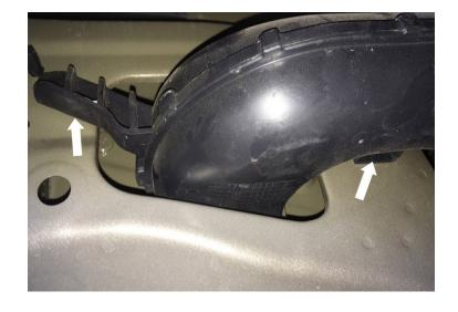
Remove the metal bushings from the stock intake box.
