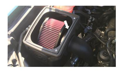
Press the Lid Seal (U) into the groove on top of the Airbox (A).
