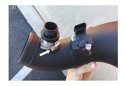
Insert the Intake Tube (C) into the Airbox (A). The intake tube stop bead should meet up to the Tube Seal (B).
