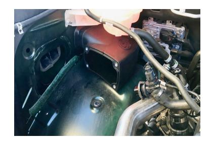
Install the Coupler (F) onto the turbo with the #44 and #52 Hose Clamps (G & H). Try to get the angle of the coupler as shown below. Tighten the hose clamp at the turbo, leave the other one loose.
