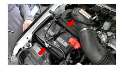
Remove the battery and battery blanket from the vehicle. The battery is heavy so be extra careful when taking it out. The battery is also filled with battery acid so remember to keep it level to prevent the acid from spilling out the top.
