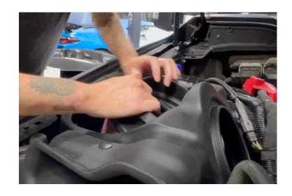
Align and center the Filter (8) with the Intake Box (1) opening. Pull the Filter flange out of the filter and use it to pull the Filter until it snaps into the opening of the Intake Box as shown in IMAGE 2. Then install the Hose Clamp (9) over the Filter flange loosely.
