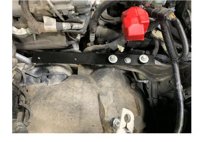
Remove the stock hold down U-bolt from the stock battery tray by first removing the two screws underneath securing the stock battery tray to the stock intake inlet.
