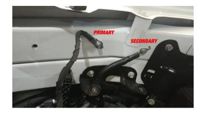
Remove the grounding bolt that attaches the primary ground to the fender. Set the grounding bolt aside to be used in Step 23.
