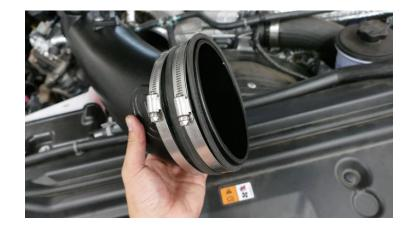
Remove the filter Hose Clamp (9) from the Filter (8), and fold the Filter flange inward towards the inside of the filter. After the Filter flange is fully inside the filter, install the Filter into the Intake Box (1).
