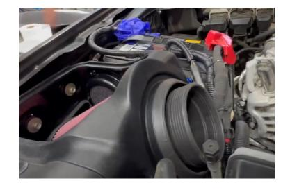
Insert a Push In Cable Tie (31), into the 1/4" hole on the Intake Box (1). Wrap the Cable Tie around the electrical harnesses and firmly secure it to the Intake Box.
