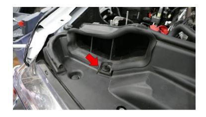
Pop-out all the wire harness clips secured to the side of the battery tray.
