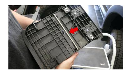
Install the stock hold down U-bolt onto the Battery Tray (22). The stock hold down U-bolt should be installed as shown. The longer end should be closest to the longer side of the Battery Tray. Use a Cable Tie (30) through the center of the battery tray to secure the hold down U-bolt.
