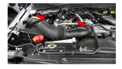
Remove the two screws securing the stock intake box.
