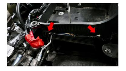
Remove the four screws then remove the battery tray from the vehicle. Set the screws aside, they will be reused in Step 14 and 35.
