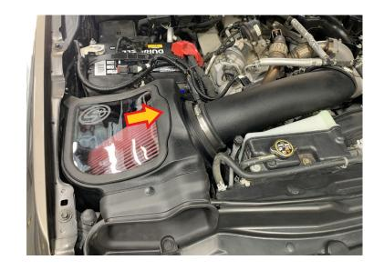
Inspect your installation, make sure the kit is properly positioned and all fasteners and hose clamps are secured. Keep all stock parts in case you would ever need to reinstall the stock intake assembly. Affix the ID label near the intake kit. If you are an installer, give the owner the QR code for the Installation Instructions so that he/she is aware of the "Periodically Check the Following" procedures given in the beginning of the Instructions. The Installation is now complete.
