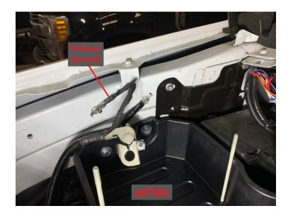
Place the battery and battery blanket inside the Battery Tray (22) as shown. Be careful as the battery is heavy. The battery is also filled with battery acid so remember to keep it level to prevent the acid from spilling out the top. Pay attention to the orientation of the battery where the negative post is closest to the fender and the positive post is closest to the engine. Also, make sure the U-bolt is on the outside of the battery blanket.
