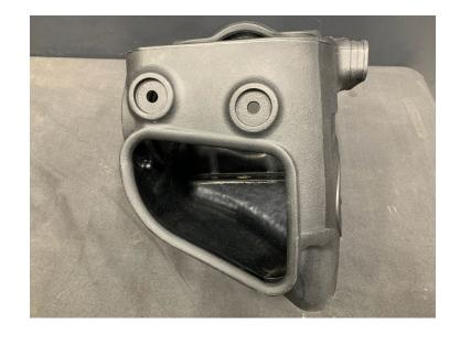
Install the Box Inlet (5) onto the Intake Box (1) with the Plastic Rivets (6). Squeeze the plastic rivets together so they interlock into place and hold the Inlet to the Box.
