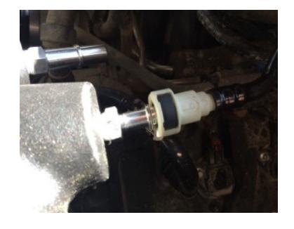
Reconnect the PCV hose. Push in the connector over the Quick Connect Fitting (Q) until you hear it snap into place.
