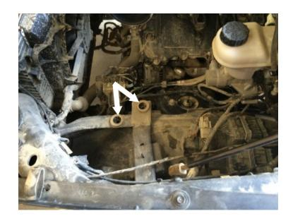
Reinstall the retaining bolt removed in Step 7 and tighten the bolt to secure the Airbox (A). Install the retaining bolt from inside the airbox.
