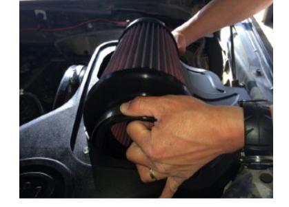
Feed the Air Intake Tube (B) underneath the coolant line through the Rubber Cuff (C) until the bead on the air intake tube meets up to the rubber cuff. Slide the Air Filter (D) over the tube until the tube bottoms out on the filter flange step.
