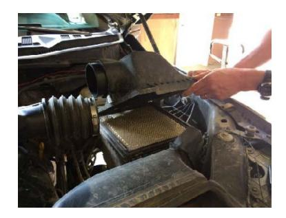
Disconnect the vacuum line. Push down on the black clip and pull the hose connector out of the hose barb.
