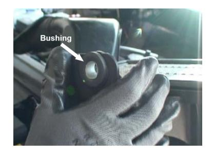
Install the grommet into Airbox (A) first and then install the metal bushing from the inside.
