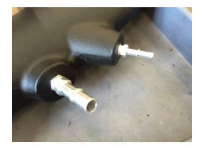
Install the Airbox (A). Make sure that the box prongs are aligned with the factory grommets. Push down on the airbox to make sure that the prongs are completely seated.
