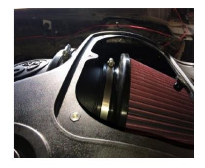
Insert the Air Intake Tube (B) into the Silicone Step Coupler (N) at the throttle body. Once everything is in place, tighten Hose Clamp #56 & #52 (O & P).
