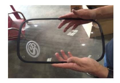
Install the Clear Lid (E) on top of the Airbox (A) and secure the lid using the six provided Truss Head Phillips Screw (M) and Sealing Washer (L). Do not over tighten.
