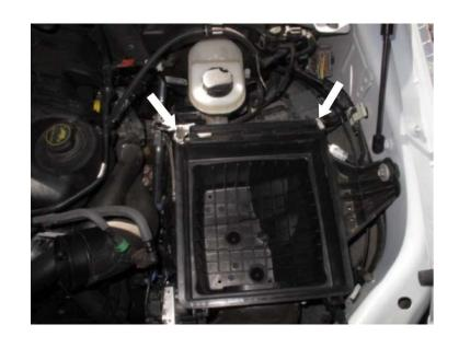
Remove the plastic rivets on the stock air scoop using a flat head screwdriver.
