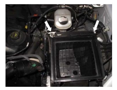
Lift and remove the stock airbox.
