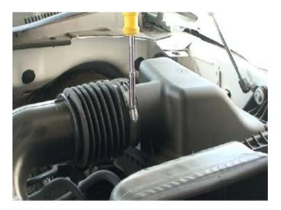
Loosen the hose clamp at the tube leading to the turbo inlet on the passenger side.
