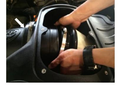
Tighten the Hose Clamp #88 (K) at the Air Filter (D).
