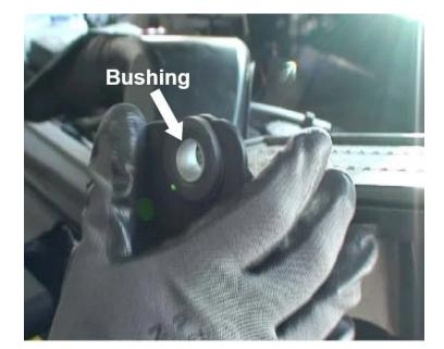
Install the grommet into Airbox (A) first and then install the metal bushing from the inside.
