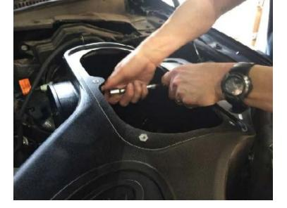
Install the IAT Sensor into the Intake Tube (B). Make sure to remove the IAT Sensor O-Ring prior to installing. Use a twisting motion to make it easier to guide the sensor into the grommet. Make sure that the sensor is seated all the way so that the sensor tab is touching the grommet and is lined up with the triangle mark located on the air intake tube.
