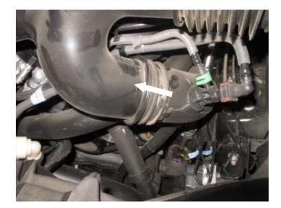
Unhook the two latches on the stock airbox.
