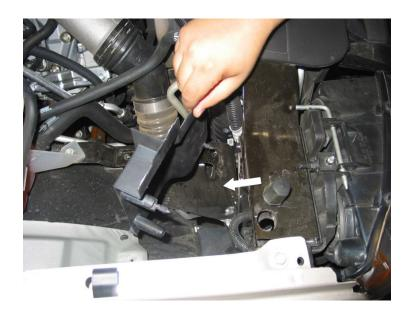
Insert the Fender Seal (R) onto the Airbox (G).
