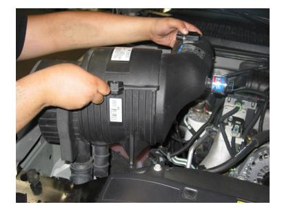
Remove the five bolts on the stock airbox tray and remove the tray from the vehicle. Be sure to save the speed clips underneath. They will be reused to install the Airbox (G) in Step 9.
