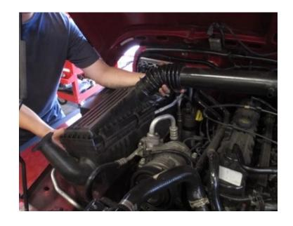
Install the Hose Barb (N) into the side of the Air Tube (H) until finger tight, then turn it one to two complete turns with a wrench.
