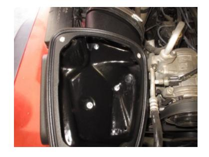
Insert the Air Filter (B) into the Airbox (A). Make sure the hose clamp is accessible. Push the connected Air Tube (F & H) through the Rubber Cuff (E) until you can slip on the air filter. Tighten the #88 Hose Clamp (L) at the air filter to secure the air filter to the tube.
