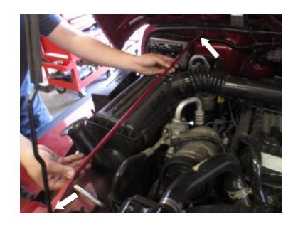
Loosen the hose clamp at the throttle body and lift the tube from the inlet.
