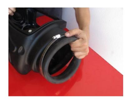
Lower the Airbox (A) as shown and align the three holes on the box with the holes on the fender.
