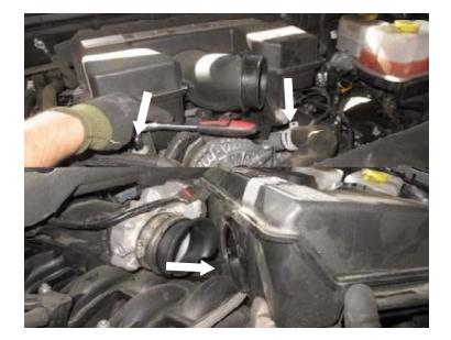
Remove the stock rubber boot from the throttle body.
