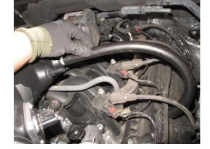
Use Hose Clamp #12 (Z) to tighten down the hose on the engine side.
