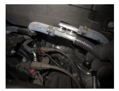
Connect the MAF Extension Harness (Y) to the vehicle connector. Zip Tie (V) away from any moving parts.
