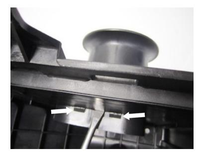
Install the Fender Inlet (J) into the factory intake box by pushing in firmly until it snaps into place.
