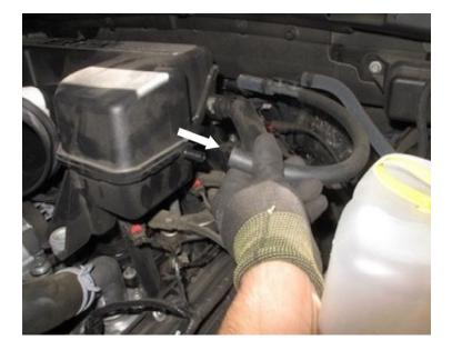
Remove the second hose from the resonator box by sliding the white tab counter clockwise to release the lock.
