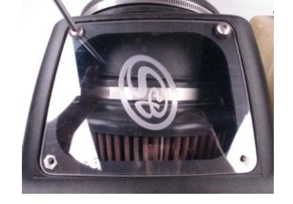
Reconnect the negative terminal on the battery. Inspect your installation, make sure the kit is properly positioned and all fasteners are secure. Affix the CARB and ID label near the intake kit. Keep all stock parts in case you would ever need to reinstall the stock intake. The installation is now complete.
