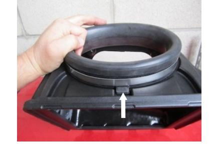
Insert the Intake Tube (H) into the Intake Box Cover (B) through the Rubber Cuff (C). Please make sure that the tube is pushed all the way to the stop bead.
