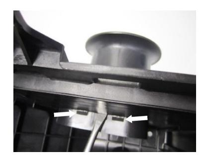
Install the Fender Inlet (W) into the factory intake box by pushing in firmly until it snaps into place.
