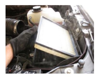
Remove the two mounting bolts securing the air intake box to get to the side air inlet. Remove the factory intake box from the vehicle.
