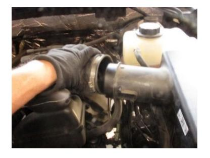
Once the hose clamp is loose, pull the factory intake tube to the left to separate from the factory intake box cover.
