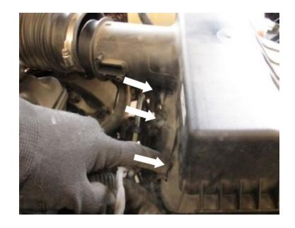
Lift to remove the factory intake box cover.
