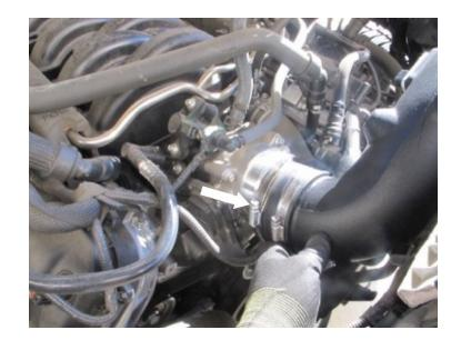
Connect the hardline from the engine to the Hose Fitting (M) and Hose (U) onto the Hose Barb (T).
