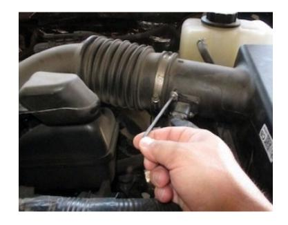
Disconnect the sensor from the harness by pulling the Red tab out and pressing down on the release button. Place the sensor in a safe location for later install.
