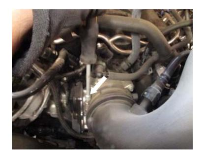
Remove the intake tube assembly from the vehicle.
