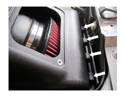
Fasten the three latches from the stock airbox.
