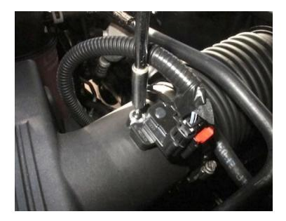
Once the sensor is removed, disconnect the sensor from the harness by pulling the Red tab out and pressing down on the release button while pulling out. Place the sensor in a safe location for later install.
