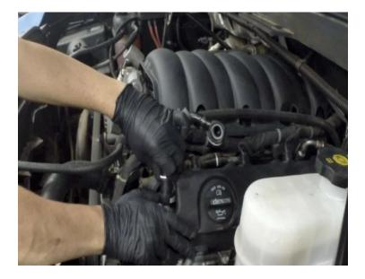
Remove the top bolt from the front crossbar using a 10mm socket.
