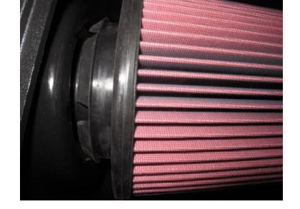
Install the larger side of the Coupler (C or D) onto the Air Tube (B) with the #72 and #64 Hose Clamps (U & T). Tighten the #72 Hose Clamp at the intake tube. The coupler used is dependent on the vehicle engine liter you have.
