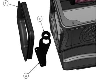
Note: If you have vehicles equipped with HID headlights proceed to Step 19, otherwise continue with Step 18. Install the Airbox (A) and remember to properly align the fender seal to the side fender opening. Secure the airbox and Filter Support Bracket (W) with the M6 Bolts (L) and Washers (K). Make sure all fasteners are tightened. Go to Step 22.
