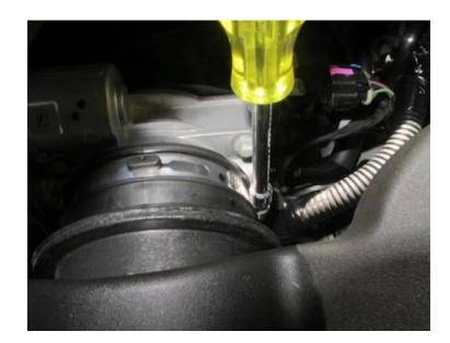
Remove the resonator box off the throttle body and out of the vehicle.
