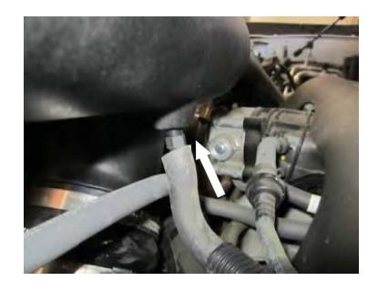
Fasten the airbox lid (P) using the provided hardware (E & F).
