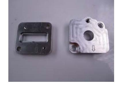
Install the adapter plate (U) or (V) and gasket (W) using the two 10-32 screws (G). Please make sure that the arrows are aligned to ensure proper installation.
