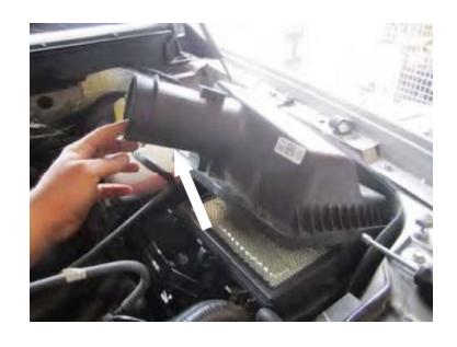
Remove the factory air filter.
