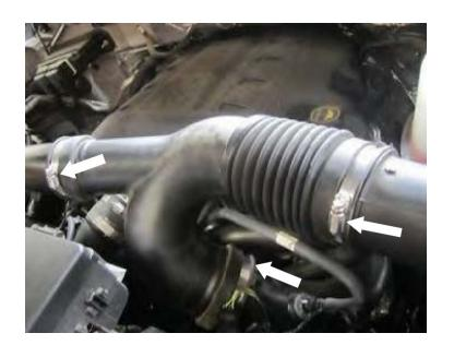
Remove the top tube by pulling out and away from the factory airbox.
