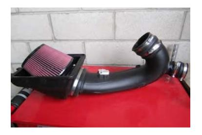
Place the whole intake assembly and lower it down into the stock intake box. Please make sure that the tabs on the S&B airbox cover fit correctly into slots on the factory box on the right-hand side. Once the tabs are in the slots lower the whole intake assembly into place.
