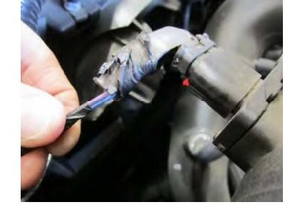
Once the sensor is removed from the tube it must be removed from the harness also.
