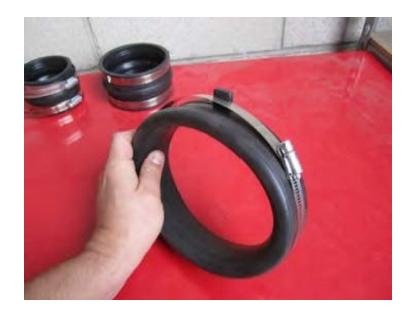
Install the cuff (R) onto the S&B airbox cover (B) making sure that the tab on the cuff aligns with the notch on the S&B Airbox Cover.
