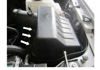
Once all three latches are disconnected lift the coverup and out to the side to remove.
