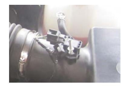
The sensor must be removed from the factory intake tube.
