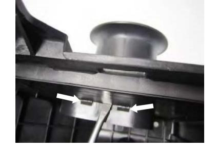
Install the S&B fender Inlet (X) by pushing in firmly, wait until it snaps into place.
