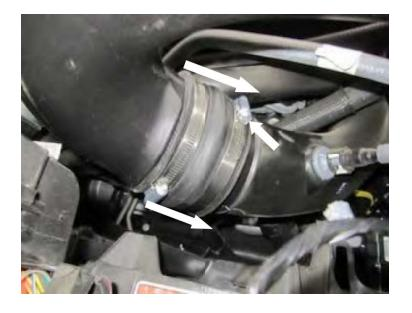
Attach the top turbo inlet tube completely and again tighten the hose clamp.
