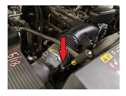
Using a suitable tool, gently pry the intake tube off the retainer clip on the coolant hose. Remove the intake tube.
