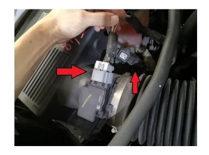
Loosen the hose clamp connecting the intake tube to the throttle body.
