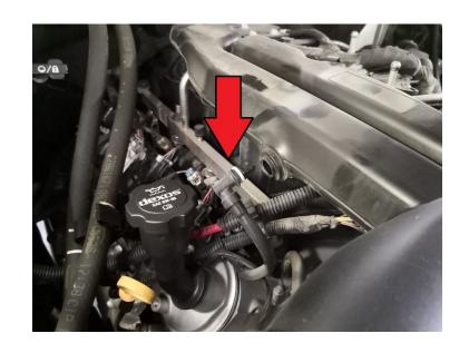
Disconnect the other end of the vent tube from the engine by sliding the locking tab over and pulling the tube to remove it.
