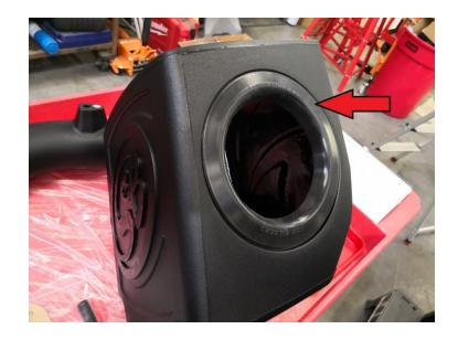
Install the airbox into the vehicle using the four M6 x 25 mm screws and washers.
