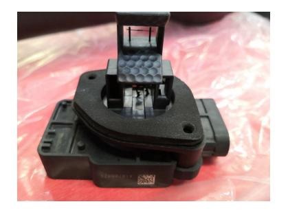
Install the MAF sensor with an adapter and gasket on to the intake tube using the #8-32 x 7/8" screws. Note: the foam gasket should be between the intake tube and the plastic adapter.
