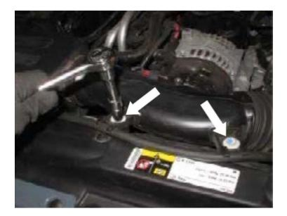
Loosen the hose clamp at the stock airbox and pull the tube out.
