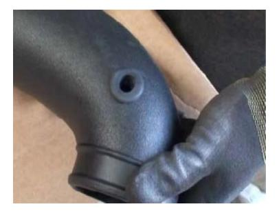
Reinstall the IAT sensor into the Air Tube (O) by pushing the sensor into the Grommet (L). Seat the sensor into the grommet until the O-ring is not visible.
