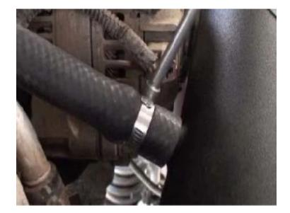
Slip the other end of the Crankcase Hose (**R**) onto the crankcase vent tube. Tighten down the #12 Hose Clamp (**S**) to secure the hose.
