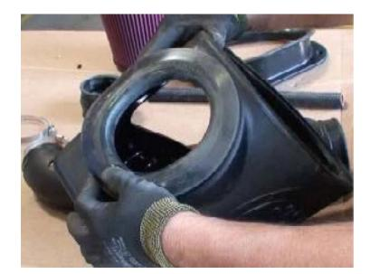
Install the Air Tube (O) into the Airbox (H) by pushing the tube through the Tube Seal (N).
