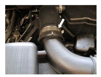
Disconnect the MAF sensor by sliding the red locking pin back, press in the bottom of the harness and pull out the male connection.
