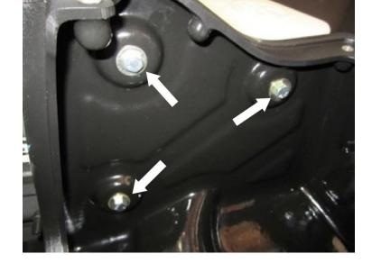
Install the Airbox/ Coolant Tank assembly into the truck. Push the prongs on the bottom of the airbox into the OE grommets set in the frame. Secure using the OE bolt removed in Step #7.
