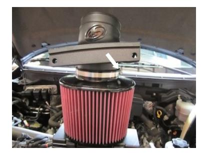
Slide the filter assembly into the Airbox. Install two #80 Hose Clamps (H) over the Hump Adapter (Q). Push the Hump hose over the end of the Adapter Tube (F).
