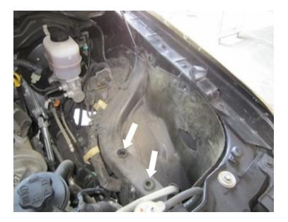
Remove the mounting insert and rubber grommet from the OE airbox assembly.
