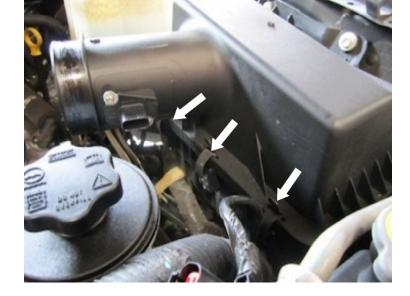
Using a 13mm socket, remove the rear airbox mounting bolt. Then carefully remove the coolant overflow tube from the reservoir and use the mounting bolt as a temporary plug for the tube.
