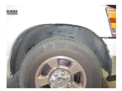
From inside the engine compartment, carefully pull the wiring harness connector out from the wheel liner. Then remove the wheel liner from the truck.
