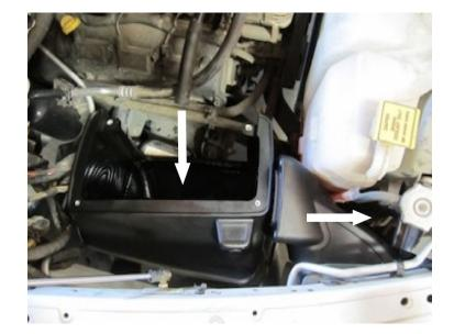
Using the OE bolt, secure the Airbox (M) to the frame. Leave loose for now.
