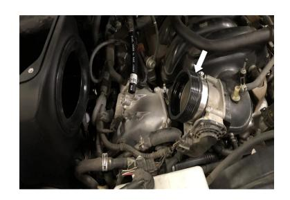
Install Intake Tube (N) by first feeding the intake tube from inside of the airbox to the throttle body and tighten Hose Clamp (S).
