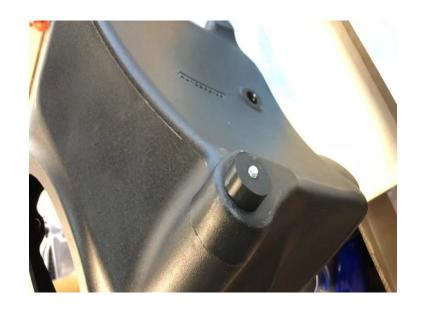
Install Tube Seal (O) onto Airbox (A).
