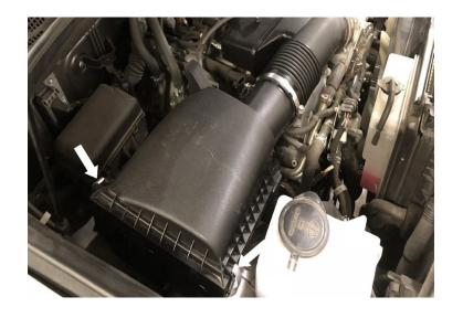
Loosen the two bolts securing the airbox and remove airbox from the vehicle.
