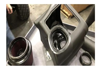
(Optional): Determine if you want to install the Box Plug (X) onto the Airbox (A). See the "Intake Box Plug" to decide the desired setup. Leave Box Plug uninstalled for maximum airflow.
