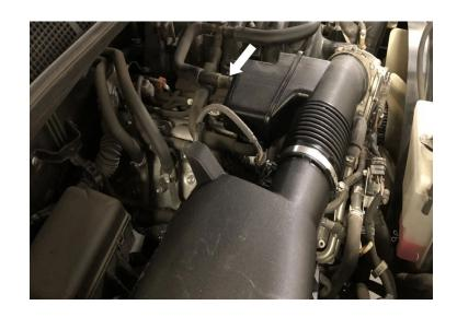
Loosen the hose clamp on the intake tube at the throttle body.
