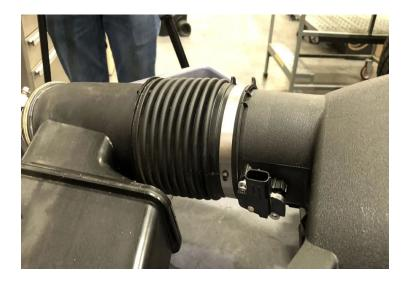
Install MAF Sensor, Plate (M), and Gasket (L) onto Intake Tube (N) with provided Hardware (P).
