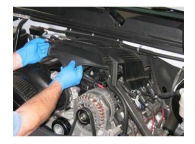
Disconnect the electrical connection to the MAF sensor at the OE airbox.
