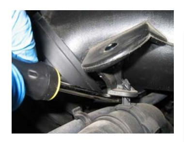
Loosen the hose clamp at the throttle body and at the MAF sensor, remove the OE intake tube from the engine.
