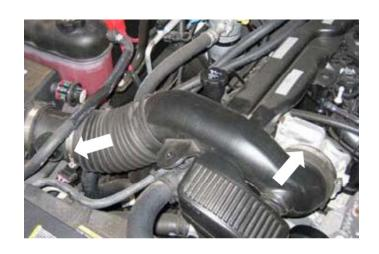
Slide the OE airbox towards the engine while pulling up, to remove from the vehicle.
