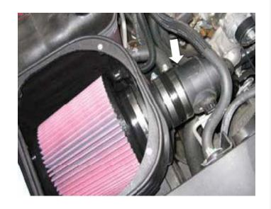
Place the S&B hump adapter (M) over the S&B tube (O), slide on until rib on the tube is captured by the groove in the adapter. Then secure with #60 hose clamp (K).
