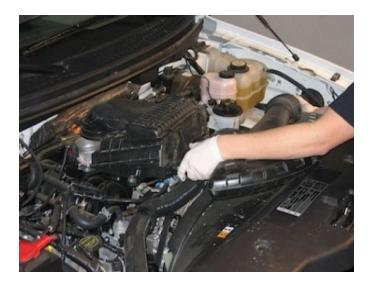
**IF EQUIPPED**: Remove the OE tube bracket only. Reinstall the lower nut on the mounting stud and tighten.
