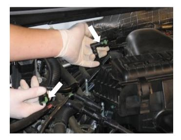
Disconnect the electrical connection for the MAF sensor, at the airbox on the Driver's side.
