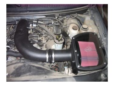
Reconnect the battery. Inspect your installation, make sure the kit is properly positioned and all fasteners are secure. Affix the CARB sticker near the intake kit. The installation is now complete.
