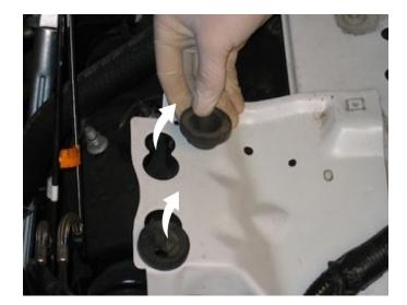
Relocate the wire loom closer to the inner fender.
