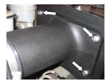
Place the Hump Adapter (H) and #72 Hose Clamp (G) over the Filter Adapter (J). **Do not tighten at his time.**
