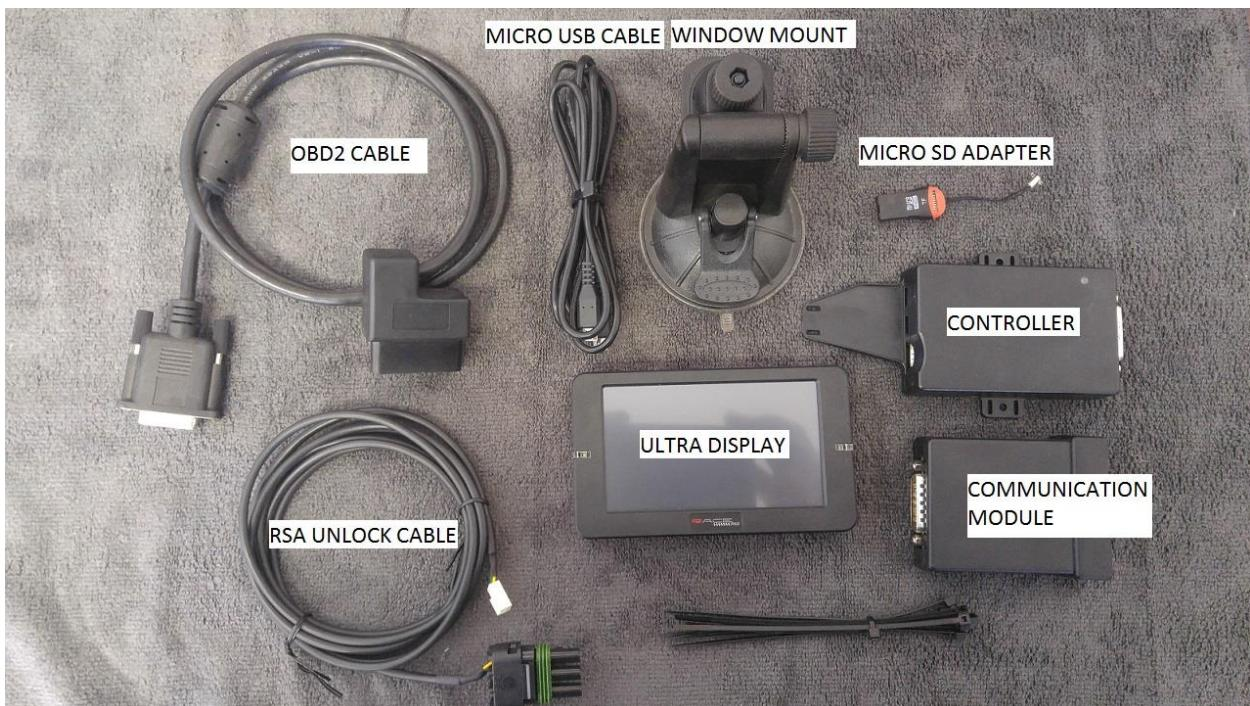
First, the Ultra display connects to the controller via the micro USB cord. Please note the orientation of the plugs to the cord as these are delicate and do NOT need to be forced.
