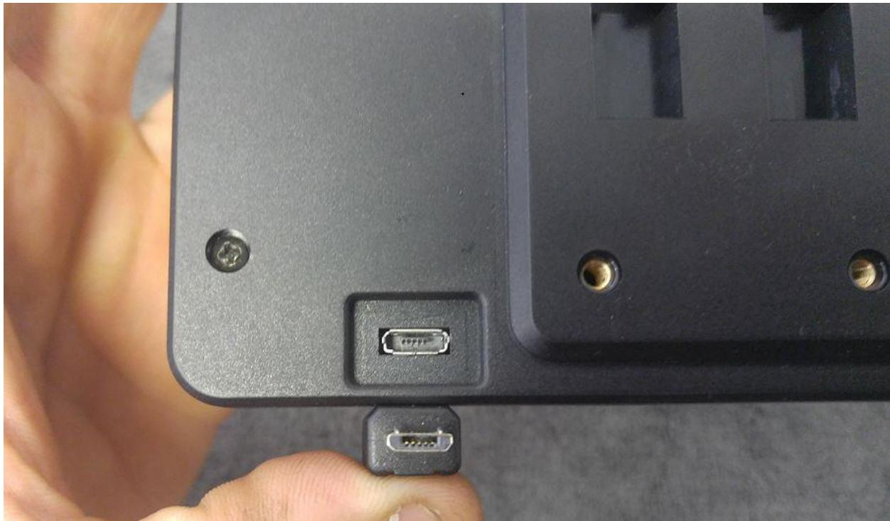
Then the controller attaches to the communication module (comm mod). These two units are press fit together.
