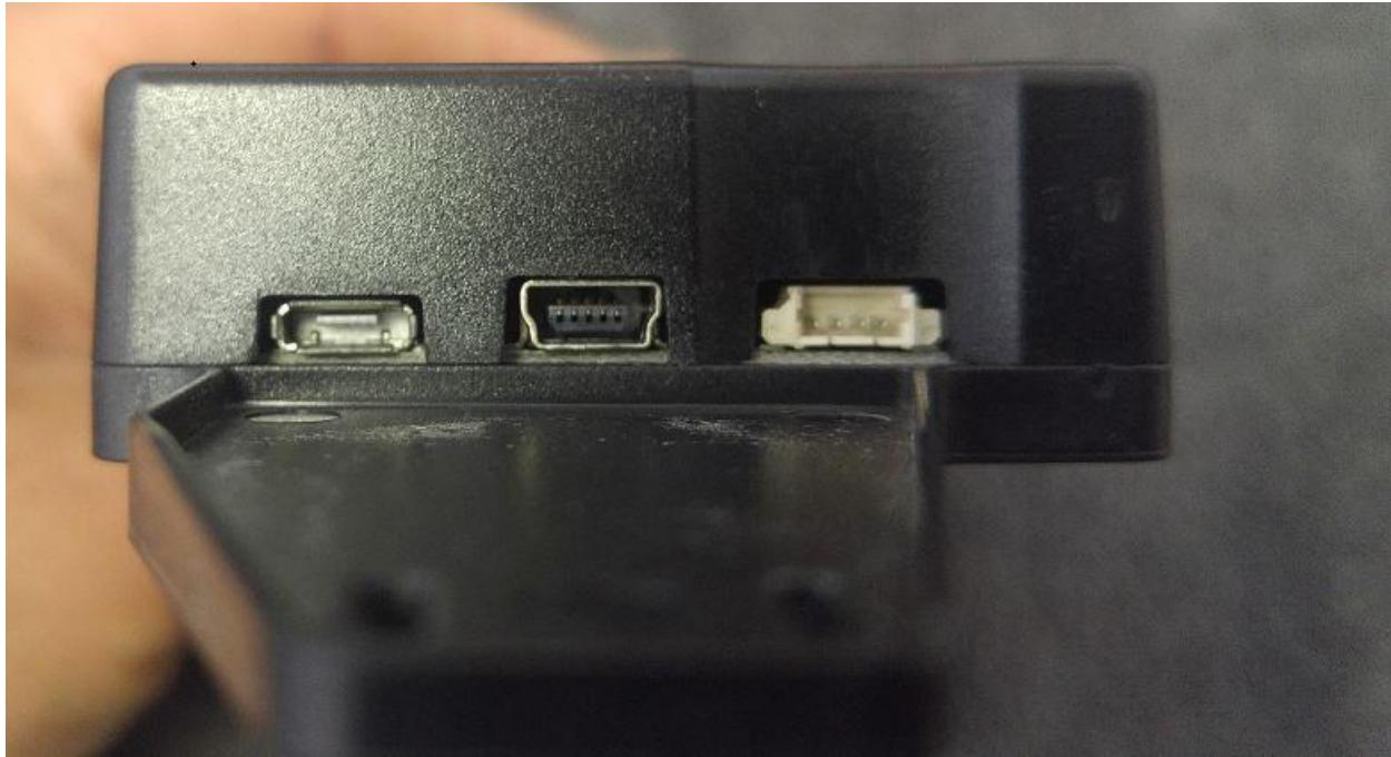
There are three ports in the end of the controller. The port on the left goes to the Ultra display. The port in the center is for remote updating with a computer. This is mostly used for custom tuners who want to make real time changes as they tune. Lastly, the port on the right is for the optional
