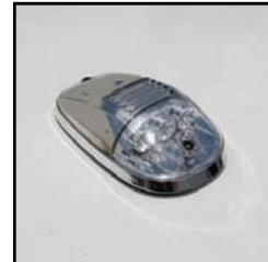
Align bolt holes in each light assembly with mounting holes in the vehicle's roof. Insert bolts removed in Step #1 and turn clockwise to finish light replacement.
