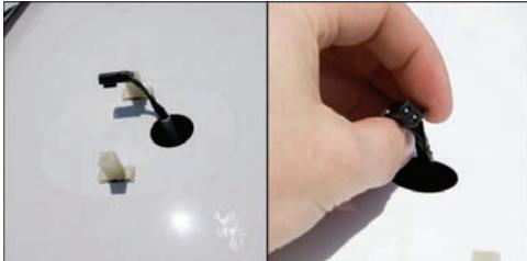
Locate the two bolts in each light and turn counter-clockwise to remove. Lift light assembly and unplug wiring. Remove light assembly completely from vehicle. Set bolts aside for later use.
