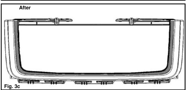
13. Position and align the **BOSS Grille** inside the factory surround. Mark the mounting locations using the brackets on the back side of the grille with a marker.
