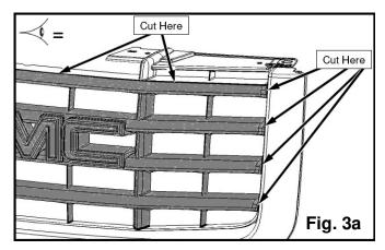
12. Carefully cut out the center section of the factory grille. Use the dashed lines in figure 3b as a guide for cutting. When you have removed the center grille section it should look like figure 3c.
