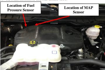
2) Remove the top engine cover, foam insulation and Air Intake tube. The top engine cover is a press-fit, it will uninstall by gently pulling up and out.
