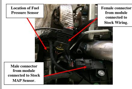
**8)** Route Switch through firewall and plug into module.
