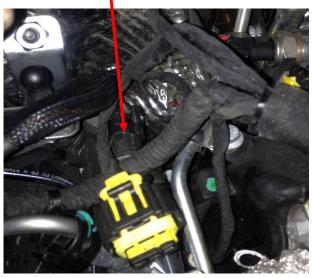
5) Connect the Stock Fuel Pressure Plug to the Female Connector from the module.
