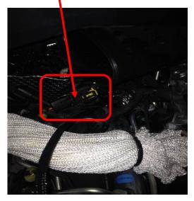
**6)** Below are photo examples representing how the factory Fuel Rail Sensor plug should be connected to our 3-Pin female connector on the ADS module harness.
