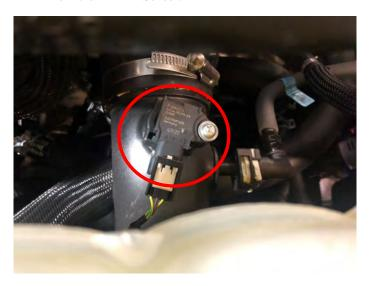
**6)** Utilize the portion of the Ag Diesel Solutions harness labeled T-MAP. Connect the male connector to the T-MAP Sensor. Then connect the female connector to the stock male T-MAP Sensor connector.
