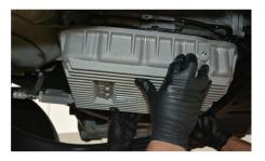
Step 5. Install remaining M6 Flat Washers and M6 Screws. Tighten in crossing pattern as depicted in Fig 1.
