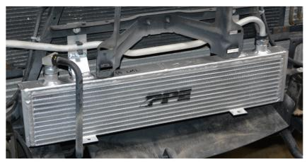
Step 15 Check fitment. Adjust as necessary.
