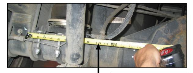
This vehicle is shown with the breather located 10" from leaf spring pack and does not require the modified breather.
