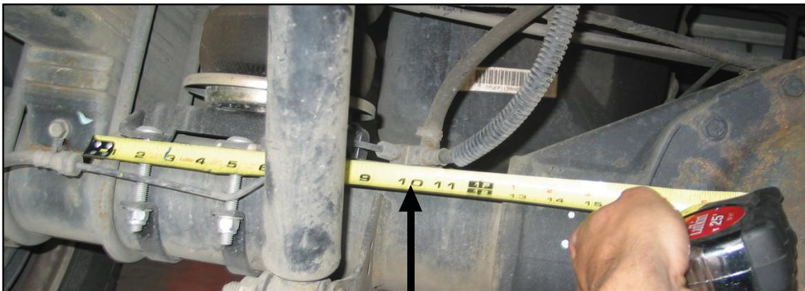
This vehicle is shown with the breather located 10" from leaf spring pack and does not require the modified breather.
