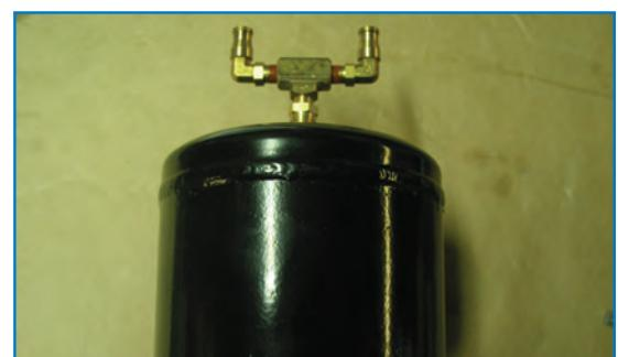
**17** Choose a location to mount the air tank such as on the driver's side bumper support brace shown in the photo. Drill two  $\frac{3}{8}$ " holes on  $3\frac{1}{4}$ " center to accommodate the tank mounting holes. Provided are two spacers and fasteners for mounting. If you prefer another location to mount the air tank, the airline provided may need to be substituted for a long piece.
