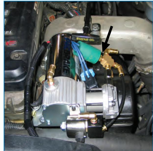
**14** Install the Black nylon airline provided to the solenoid port marked "CYL". Route this airline around the front of the engine to the exhaust brake air cylinder, keeping it away from heat sources and moving parts. Install the 90° fitting supplied into the air cylinder using thread sealant and connect the airline. Cut the airline to length with a sharp razor knife. Secure the airline with the tie-straps provided.
