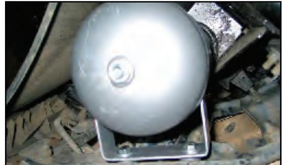
**18** Connect the Black nylon airline to the remaining fitting at the compressor. Route it to the top of the air tank. Cut the airline to length with a sharp razor knife. Connect the  $\frac{1}{4}$ " airline to either fitting in the tank. Secure the airline away from moving parts and heat sources using the tie-straps provided.
