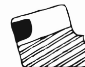
ILLUSTRATION: E INCORRECT PATTERN (DRIVE SIDE)
