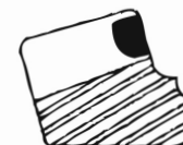
ILLUSTRATION: D INCORRECT PATTERN (COAST SIDE)
