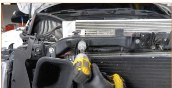
07. Remove the bolt that secures the AC condenser support.
