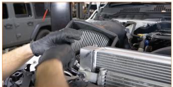
**11.** Pull the spring clip on the passenger-side transmission cooler line.
