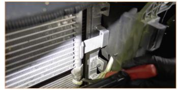
**12.** Do the same for the driver side. Pull the spring clip to free the line and then separate the line from the cooler. (1x spring clip)
