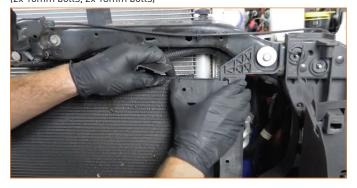
23. Reattach the shrouding on both sides of the AC condenser.(6x pop-clips)
