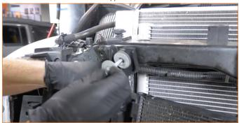
22. Reinstall the AC condenser, including the brackets on the driver side.(2x 10mm bolts, 2x 13mm bolts)
