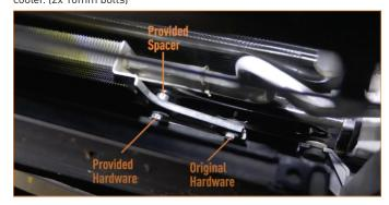
21. Reinstall the AC condenser support. (1x 13mm bolt)
