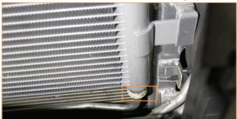
18. On each side of the cooler, use the provided long bolt and place it
