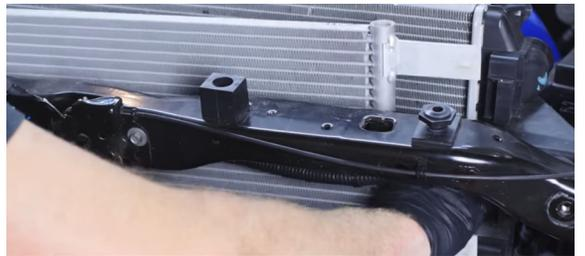
23. Pull the rubber bushings off the radiator brackets.
