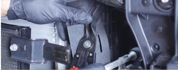
17. Compress the clamp securing the top radiator hose to the radiator, and slide the clamp down the hose. Then, separate the hose from the port on the radiator. (1x spring clamp)
