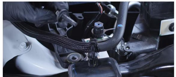
4. Separate the top portion of the airbox from the bottom. (8mm screws or plastic clips)
