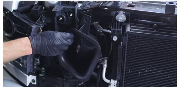
14. Loosen the AC condenser from the plastic bracket on the passenger side. Then, slide the condenser over to separate it from the tabs on the opposite side bracket. Let the condenser rest in place. (3x 13mm bolts)
