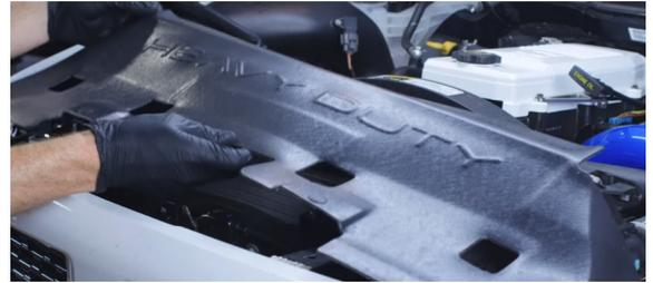
2. Four bolts hold up the front grille. Unscrew those bolts and lift the front grille from the vehicle.
