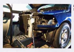
**Figure 8**: Dynamometer testing of the Mishimoto Intercooler
