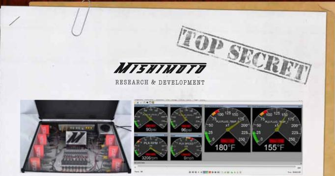
Air intake temperatures (AIT) were taken from the inlets and outlets of both intercoolers using PLX K-type thermocouples. Boost pressure was also tested to ensure that no dramatic pressure drop occurs when installing the larger Mishimoto intercooler.
