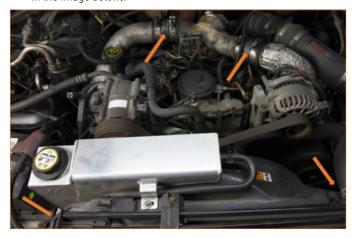
04. Using the Mishimoto supplied boot kit, attach the appropriate boots to their corresponding locations. This bead should go onto the intercooler pipe.
