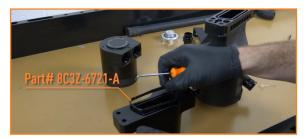
7. Attach the fitting and oil fill cap to the Mishimoto oil fill. Tighten the fitting with an adjustable wrench.
