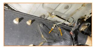
16. Install the bracket and catch can where you just removed the bolt and nut. Make sure to replace the ground strap over the bracket.
