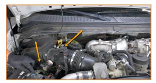
Remove the bolts that secure the airbox. (2x 13mm bolts)
