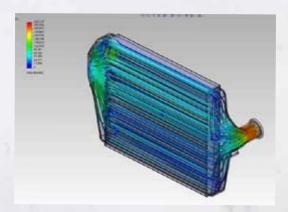
The engineering team went through multiple iterations while designing the end tanks. They used CFD software to make sure that the flow was optimized for the Ford F-250. The core of the Mishimoto intercooler is 33% thicker and 32.5% larger in volume than the stock unit. The Mishimoto intercooler has casted end tanks and a bar-and-plate core, versus the tube-and-fin core and plastic end tanks of the stock unit.
