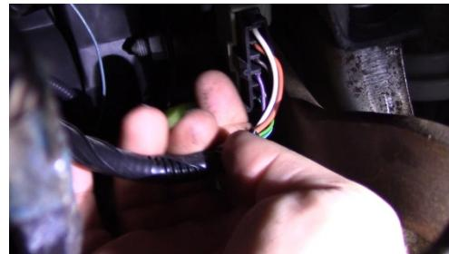
20. Locate and unplug the connector on the brake switch. It is directly above the top of the brake pedal.
