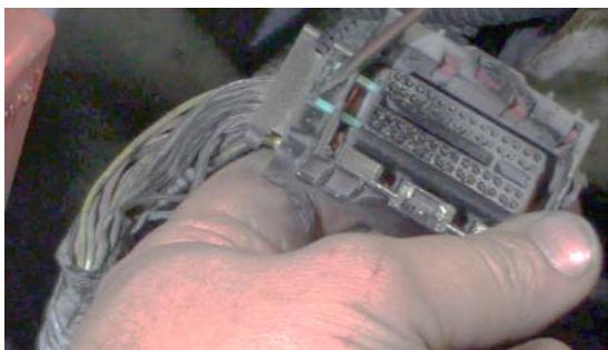
6. Remove the terminal retainer from the connector body by using a small screwdriver to remove it and slide it out
