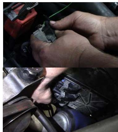
12. Reinstall the plastic cover on the connector and hook the connector back up to the ECM.
