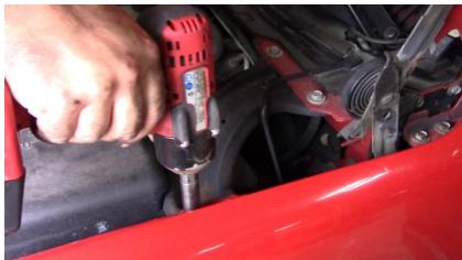
14. Up at the fire wall remove the fender brace.
