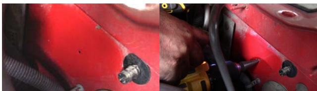
17. Locate the dimple in the firewall. Drill a hole at the dimple to fit the supplied grommet. Deburr hole. Install grommet.
