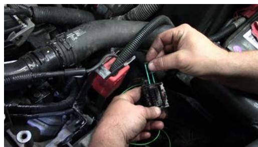
10. Reinstall the terminal retainer into the connector body
