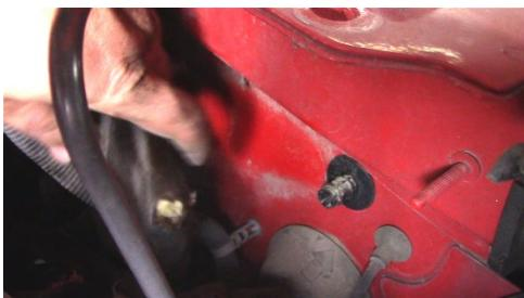
16. Remove the clip and pull back the fire wall insulation.
