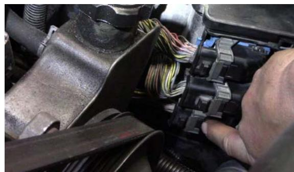
4. Locate the lower connector as mounted on the ECM. This is the C3 Connector. It has a grey body. To release the connector, push in on the center tab and pull on the grey lever.
