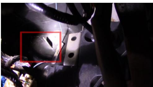
18. From inside the truck on the fire wall, locate the removable tab. Remove the tab and the insulation behind it.
