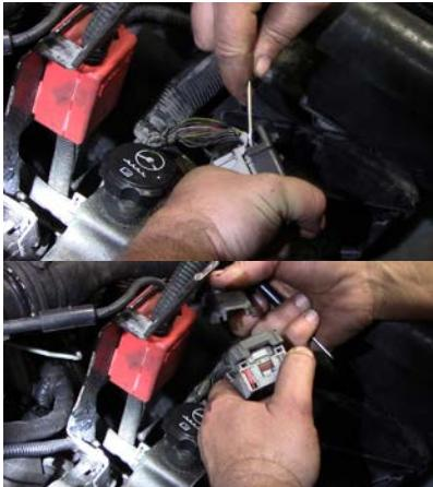
5. Remove the cover over the top of the connector exposing the wires and cut the zip tie holding the wires to the connector body
