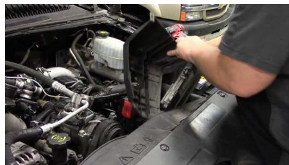
2. Release the tabs holding the TCM into the cover. Set cover aside.
