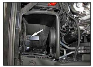
8. Install the heat shield assembly into the vehicle and secure it to the inner fender with one of the factory bolts from step #5 where shown.
