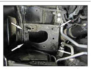
5. Remove the four bolts that secure the air filter housing mounting plate to the inner fender and then remove the mounting plate from the vehicle. NOTE: Three of the factory bolts will be reused in a later step.
