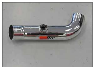
12. Install the mass air sensor into the K&N<sup>®</sup> intake tube and secure with the provided hardware.
