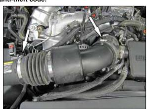
2. Loosen the two hose clamps that secure the intake tube to the air filter housing and intake plenum, then remove the intake tube from the vehicle.
