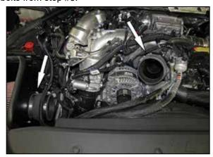
10. Install the two provided hump couplers (08418) onto the filter adapter and turbo inlet and secure with the provided hose clamps.
