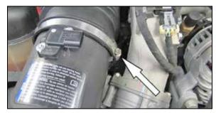
3. Loosen the hose clamp securing the factory intake tube to the air box.
