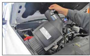
5. Lift up and remove the air filter assembly from the vehicle.
