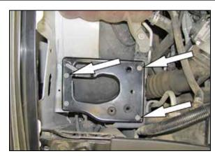
6. Remove the three bolts shown securing the air filter mounting plate.
