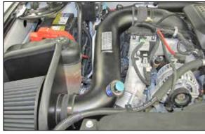
17. Install the K&N® intake tube into the hump hose at the turbo inlet and then into the hose at the filter adapter. Align the tube for best fit and then secure with the provided hose clamps.
