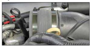
15. Install the provided hump hose (08617) onto the turbo inlet and secure with the provided hose clamp.
