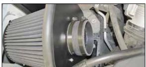
16. Install the provided coupling hose (08761) onto the filter adapter and secure with the provided hose
