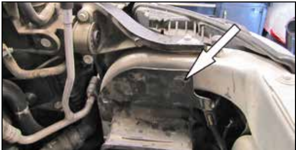
16. Remove the push pin securing the top of the fresh air intake duct.
