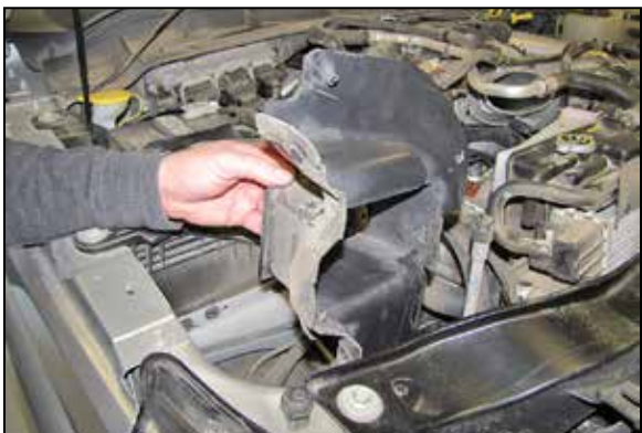
18. Remove the fresh air intake duct from the vehicle. Secure the inner fender to the vehicle with the original hardware from step #15.
