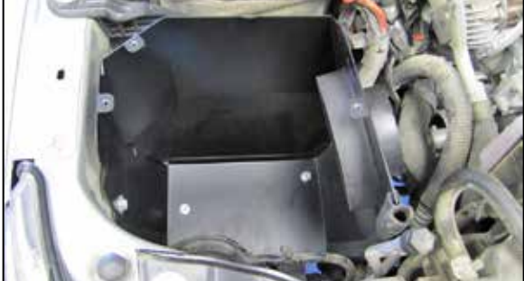
23. Set the heat shield assembly into position and secure with the factory mounting hardware from step #12.
