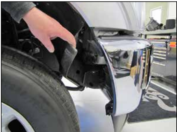
14. Remove the 5 bolts and one push pin securing the front of the inner fender panel and then pull the inner fender panel back to gain access to the bottom of the fresh air intake duct.
