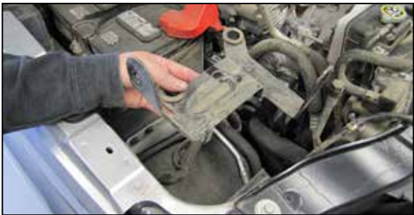
12. Remove the air box mounting bracket from the vehicle.
