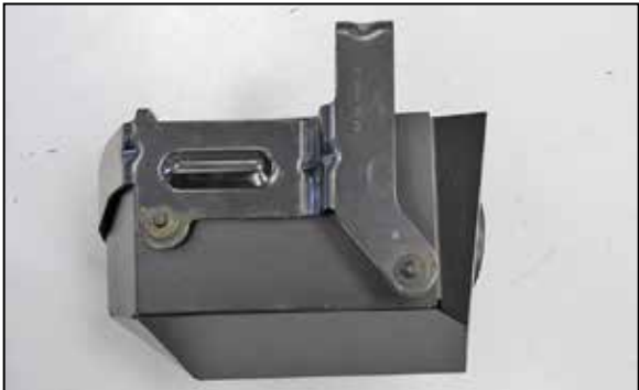
21. Install the factory air box mounting bracket onto the heat shield as shown so that the mount stand-offs installed in step #20 snap into the factory mounting grommets.
