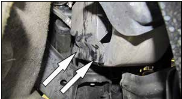
15. Remove the two clips shown that retain the bottom of the fresh air intake duct.
