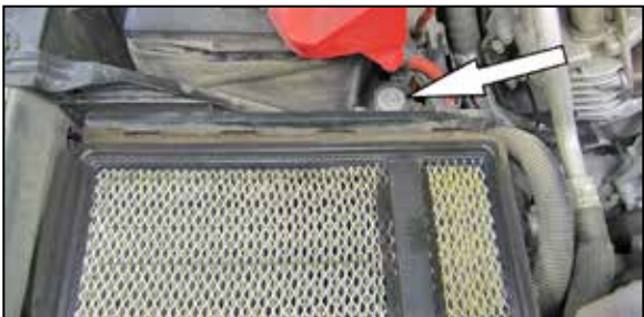
9. Remove the bolt securing the lower air box to the battery tray.
