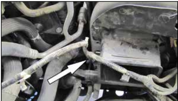
17. Unhook the wiring harness secured to the core support through the fresh air intake duct.
