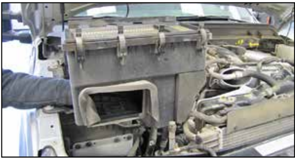
10. Remove the lower air box from the vehicle. NOTE: K&N Engineering, Inc., recommends that customers do not discard factory air intake.
