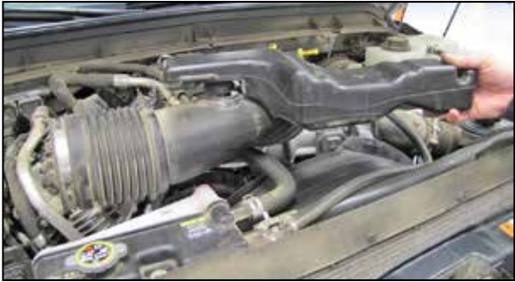
8. Loosen the hose clamp which secures the intake tube to the engine inlet then remove the intake tube from the vehicle.
