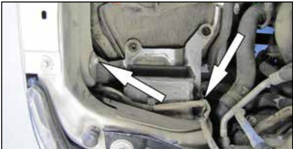
11. Remove the two bolts which secure the air box mounting bracket to the core support and inner fender.
