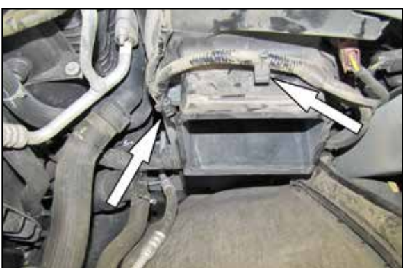
13. Unhook the wiring harness from the fresh air intake duct.
