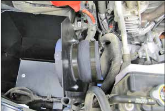
24. Install the silicone hump hose (08418) onto the filter adapter and secure with the provided hose clamp.
