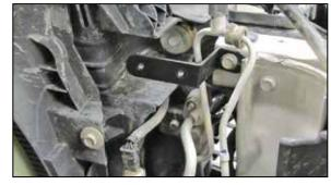
8. Install the air box mounting bracket (083145) onto the core support using the bolt removed in the previous step.
