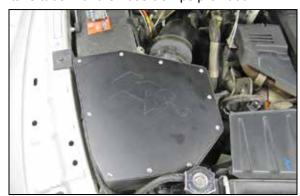
18. Install the air box lid and secure with the provided hardware.
