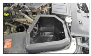
11. Install the air box so the mounting studs insert into the air box mounting grommets and then secure the air box to the mounting bracket installed in step #8. Tighten the mounting bracket bolts.
