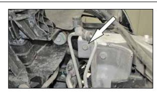
7. Remove the core support bolt shown. **NOTE: This bolt will be reused in the next step.**
