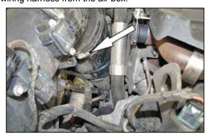
3. Loosen the hose clamp which secures the intake resonator to the turbo inlet hose.
