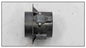
13. Install the mass air sensor and map sensor into the K&N® mass air sensor housing using a twisting motion to aid installation and then secure with the provided hardware.
