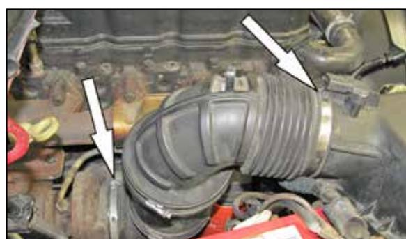
3. Loosen the hose clamps securing the intake hose to the turbo inlet and to the factory air box.
