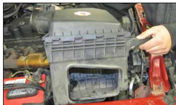
6. Lift up the air box to dislodge it from the mounting grommets and then remove the air box from the vehicle.
