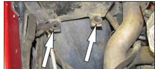
7. Remove the two air box mounting grommets from the mount.
