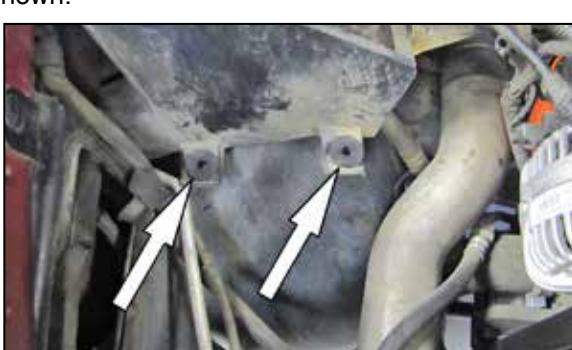
14. Install the two provided inserted nuts into the air box mounting grommet locations.
