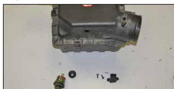
17. Remove the inlet air temperature sensor. On vehicles equipped with a filter minder, remove the filter minder and grommet from the air box.
