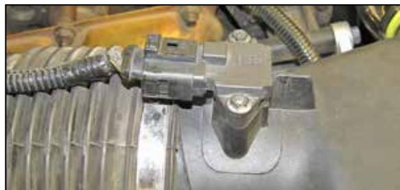
2. Disconnect the inlet air temperature sensor electrical connection.
