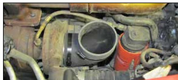
16. Install the provided 90° hose onto the turbo inlet and secure with the provided hose clamps. **NOTE: Do not completely tighten the hose clamp at this time.**
