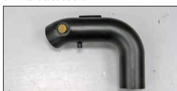
19. On vehicles equipped with a filter minder, drill a 5/8" id hole 6" from end of tube and then install the factory filter minder and grommet.
