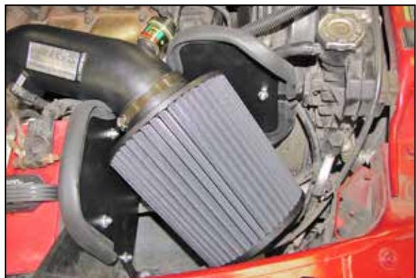
21. Install the K&N® air filter onto the K&N® intake tube.
