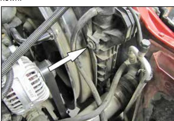
13. Remove the factory fan shroud retaining bolt shown.
