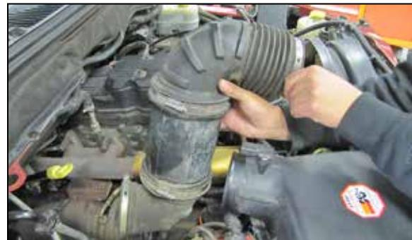
4. Remove the intake hose from the vehicle.
