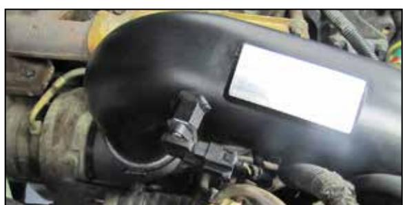
22. Reconnect the inlet air temperature sensor electrical connection.
