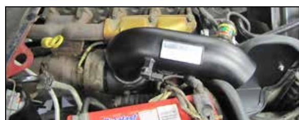
20. Install the K&N® intake tube into the silicone hose installed during step #16 and align with the mounting bracket installed onto the heat shield. Adjust the hose and tube for proper fit and then secure the hose and tube with the provided hardware.
