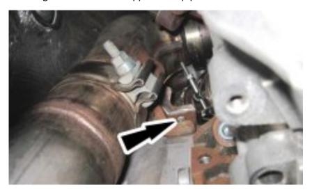
4. Install the new exhaust lower downpipe-to-catalyst and particulate filter assembly bolts and hand tighten.
