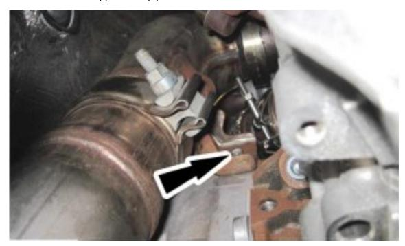
10. Remove the 2 exhaust lower downpipe-to-catalyst and particulate filter assembly bolts and remove the downpipe assembly.
