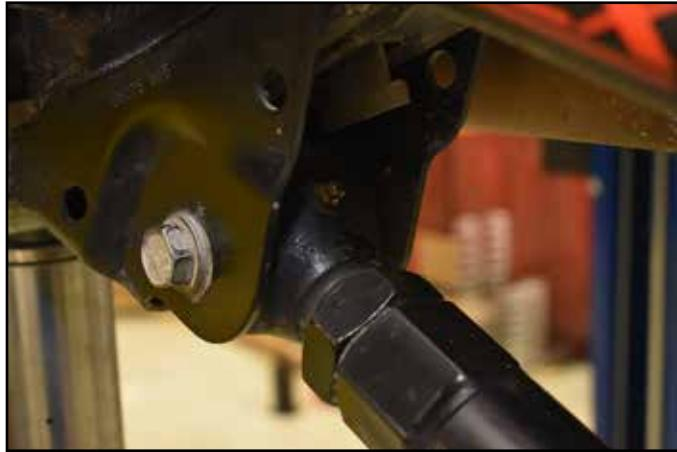
**HINT:** If mounting bolt is difficult to install due to misalignment of the control arm bushing with mounting bracket, either (1) adjust height of axle housing with hydraulic jack,
