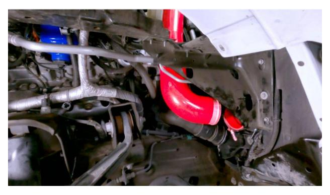
16. Slip the lower hose on, be sure it slides in far enough for the clamp to clear the bead.
