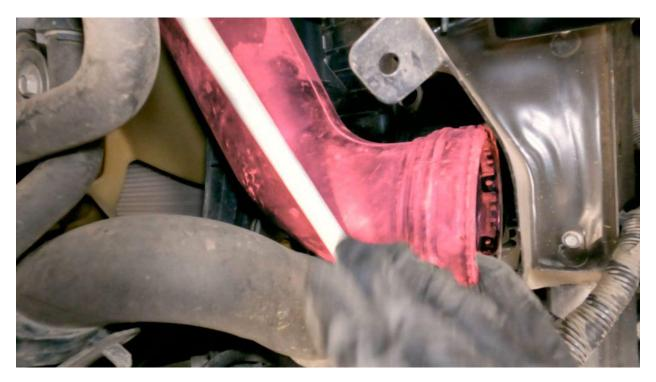
7. Rotate and free the OE cold side boost tube.
