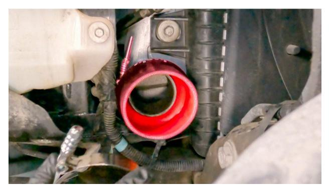
6. Slide the smaller end of hump hose #94511 with a 3-1/2 inch clamp (#92895) onto the Charge Air Cooler.
