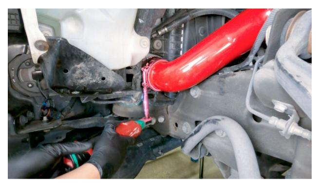
13. Slip the lower hose onto the Boost tube. Be sure it slides in far enough for the clamp to clear the bead. Tighten to 5-ft/lb.
