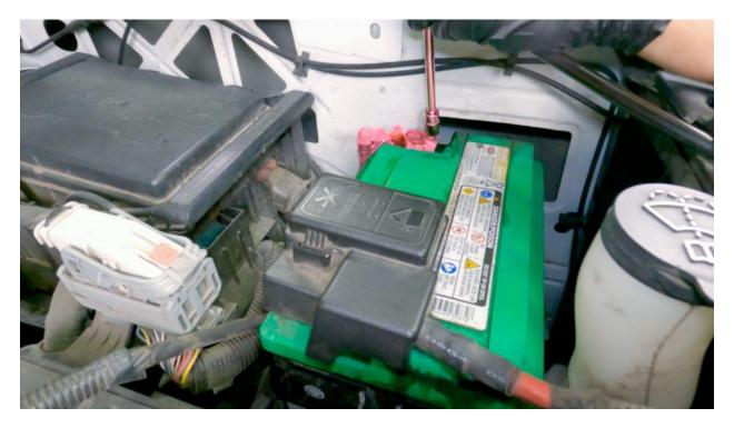
3. Using a 10mm socket, loosen and remove the negative terminal on the driver's side battery.
