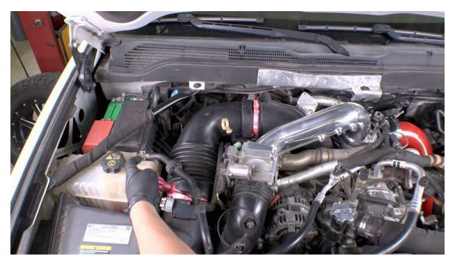
1. Start by loosening the two clamps on the factory intake tube.
