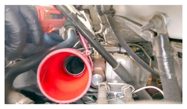
8. Slide the smaller end of the Banks Turbo Outlet Hose (#94299) and 2-1/2 inch clamp (#92852) onto the turbo outlet.
