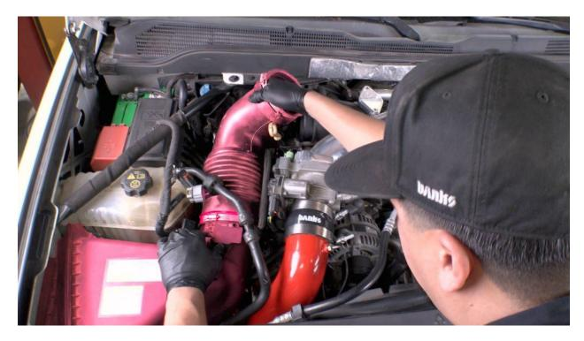
20. Drop in and re-install the air intake system.
