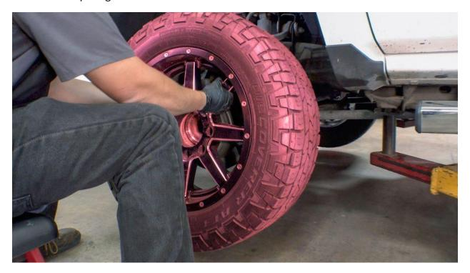
1. Secure the truck on a lift and remove both front wheels to allow for full access.
