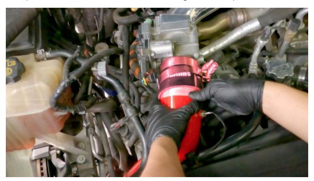
17. Slip the hose onto the top of the Boost Tube. Be sure it slides in far enough for the clamp to clear the bead.
