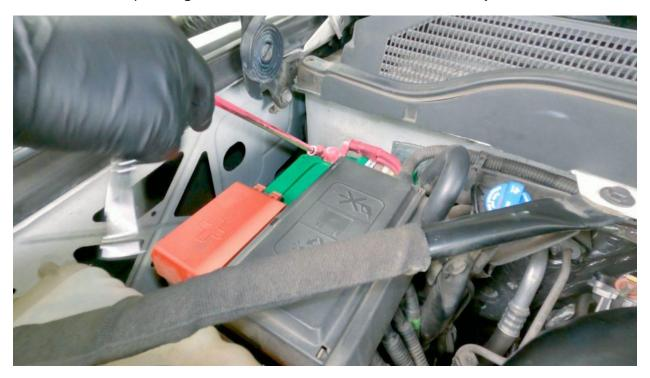
Section 1: Removal of the OEM hot side tube
