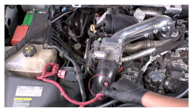
3. Unplug the 3 Air Intake Sensors on the factory air box and cold side boost tube.
