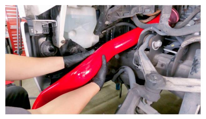
10. From underneath the truck, work the Banks Driver Side Boost Tube up through the wheel well.
