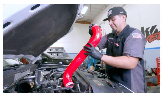
15. From the top of the truck, slide the Banks cold side Boost Tube down and into position with the lower cold side hose.
