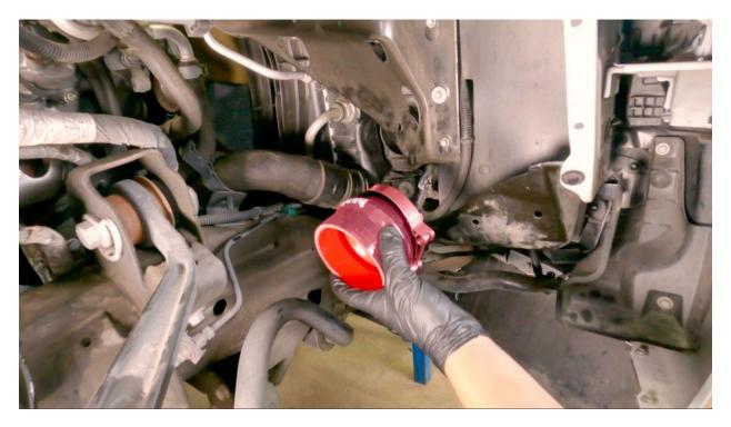
10. Slip the smaller end of the lower cold side hose (94311) and 3.78" Clamp (92899) onto the charge air cooler outlet.
