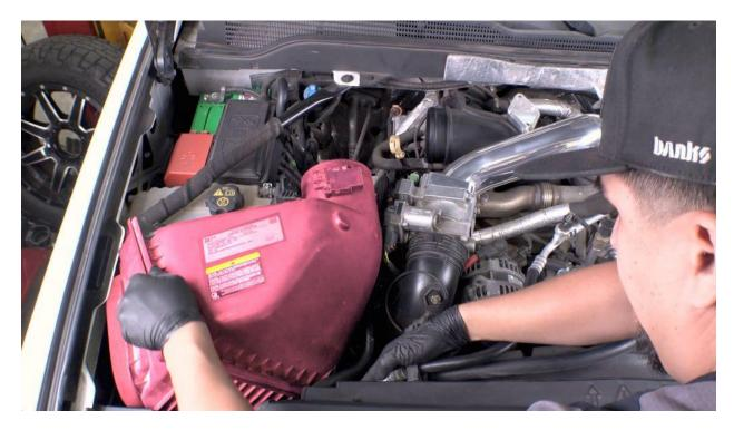
4. Lift up and remove the factory airbox from the truck.
