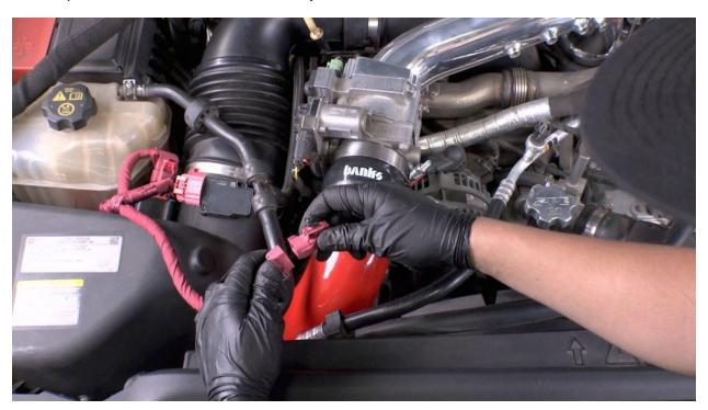
19. Plug in the 3 air intake sensors.
