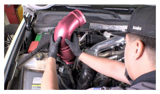
2. Lift and remove the factory air intake tube from the truck.
