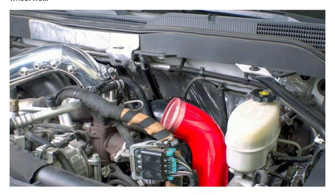
11. Rotate the tube until the top can slip into the turbo outlet hose.
