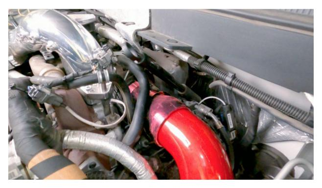
12. Be sure the turbo outlet hose slides over the tube far enough for the clamp to clear the bead.
