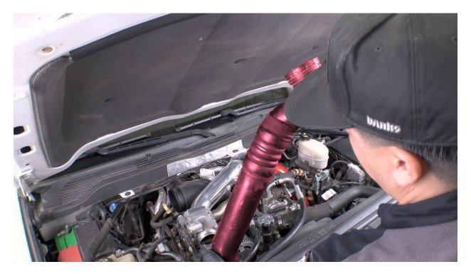
8. Remove the Cold-Side Boost-Tube through the top of the truck.
