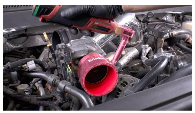
13. Slip the smaller end of the throttle body hose (94312) and 3.5" clamp (92899) onto the throttle body. Tighten to  $5\,\mathrm{ft/lbs}$
