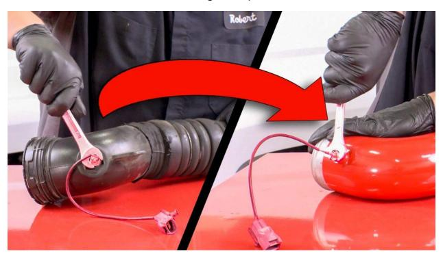
9. Transfer the Intake Air Temp sensor to the Banks Cold-Side Boost-Tube
