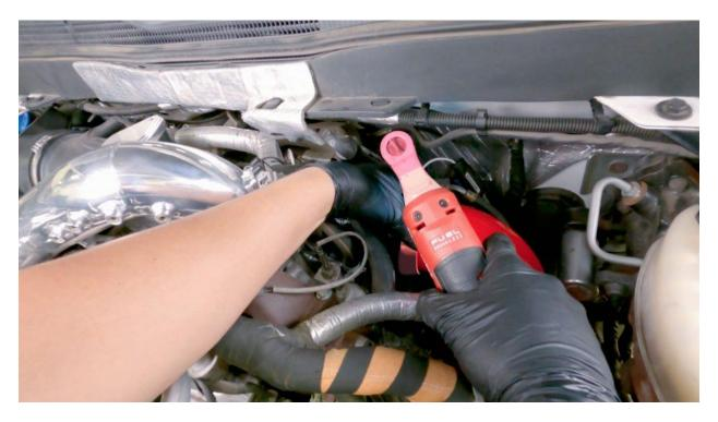
14. With the lower clamps secure, return to the top clamps and tighten to 5-ft/lb.
