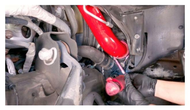
18. Adjust the Boost Tube as needed for fitment, and be sure the beads are fully seated into the hoses before tightening the clamps to 5 ft-lbs.
