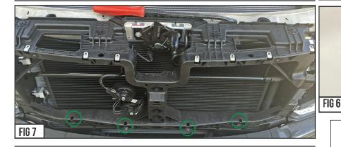
Note the location of the where the Factory Grille is fastened to the vehicle's core support.
