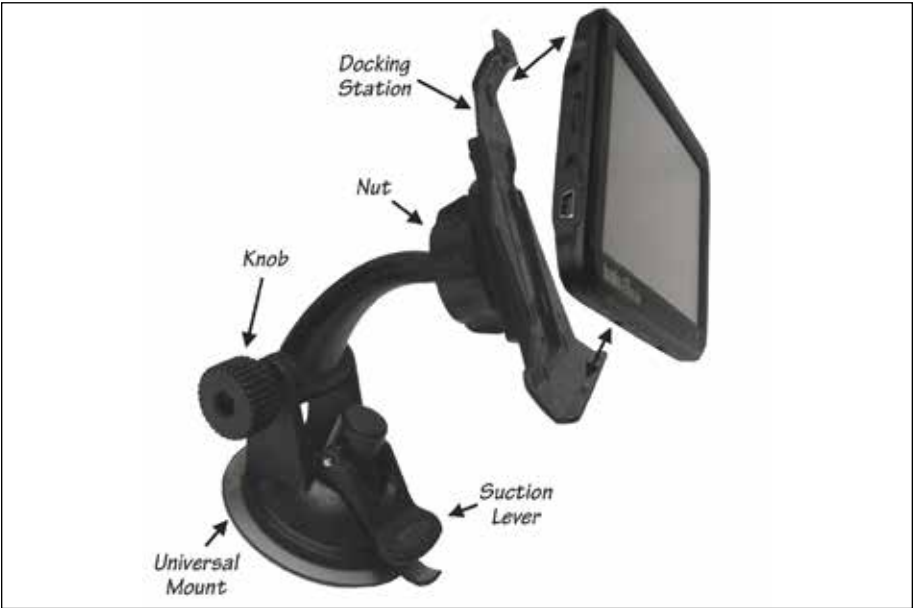
Figure 3 Attaching Banks iDash to window mount
