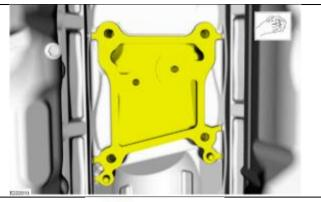
2. Ensure turbocharger pedestal bolts are tight and torqued to 26 lb ft (35 Nm)
