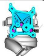
3. Install the turbocharger and loosely install the mounting bolts.
