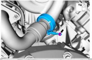
5. Tighten the new turbocharger mounting bolts in the following sequence.
