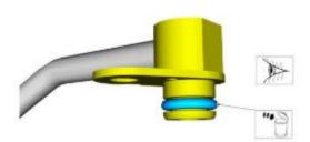
8. Loosen off and remove the turbocharger mounting bolts.
