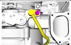
8. Install the turbo downpipe.
