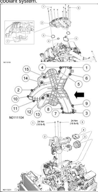
3. Remove turbocharger heat shield. 4. Remove and inspect the CAC tube for debris. 5. Remove the exhaust downpipe. 6. Remove the turbocharger inlet pipe clamps.
