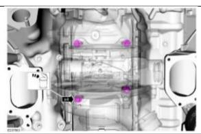
9. Remove the turbocharger.
