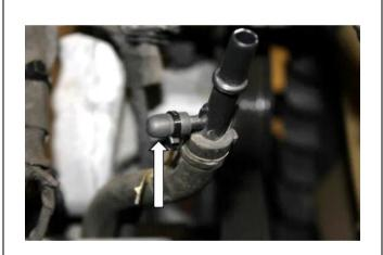
6. Remove the turbocharger coolant outlet tube.
