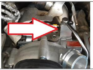
11. Disconnect the turbocharger actuator electrical connector and disconnect the wastegate actuator vacuum hose on pickup models.
