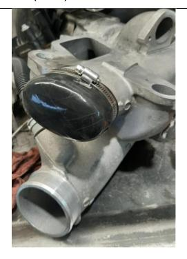
Install the upper and lower intake manifold assembly.
