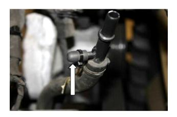
12. Pickup Trucks: plug in harness 1515950 into the wastegate solenoid harness and in-line with the exhaust back pressure sensor.
