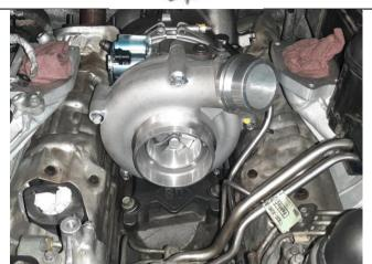
5. Connect hot-pipe feed tubes and lightly tighten v-band clamps.
