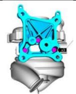
4. Use gasket BC3Z-6587-A and insert turbocharger.
