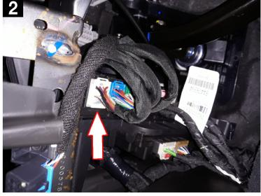
3. Plug the female end of the In-Line Speedometer Calibrator Module harness into the white plug of the Body Control Module (BCM). Ensure the connector is fully seated and locked into place.
