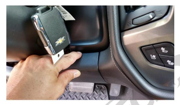
4. There is a small module with 2 connectors, underneath the dash on the left side, above the emergency brake pedal. This will be in front of a larger module with several connectors. We will be removing the black connector. With a pick or small screwdriver, slide the red locking clip backwards and depress the tab on top while pulling back to remove the connector.
