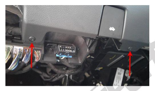
3. Pull down on the top of the Kick Panel on the left and right side to detach the clips. Once disconnected place it in the floorboard, disconnecting the hood release is not necessary.
