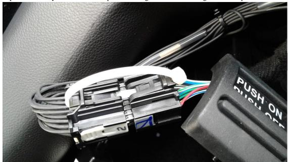
6. Connect the female end of the Speedometer Calibrator harness into the vehicle's module.
