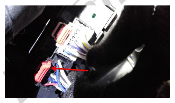
5. Plug the male end of the Speedometer Calibrator harness into the factory harness, making sure to align the retaining clips so that they are both facing up. Insert a zip tie through the retaining clips for security. Be sure not to pull it too tight to avoid damage to the clips.
