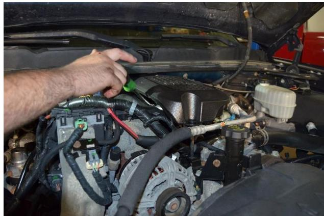
3. Remove the 10mm bolts holding the PCV hose assembly to the valve covers. The one on the drivers side will be hidden under the bail connectors
