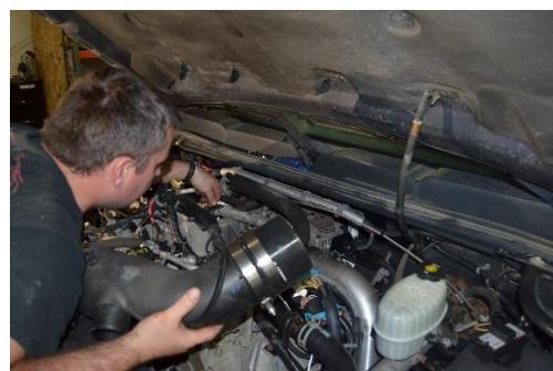
6. Clean any oil and debris from the inlet of the turbocharger and V-band clamp using a rag and degreaser. Be sure not to allow any of the debris into to the turbocharger.
