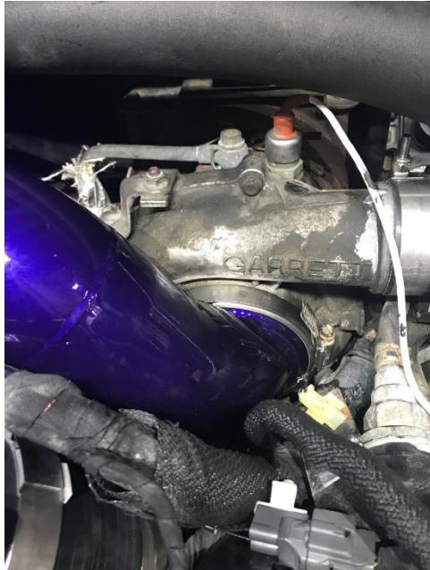
8. Tighten the V-band and intake clamps, and then reconnect the VGT actuator and wiring harness.
