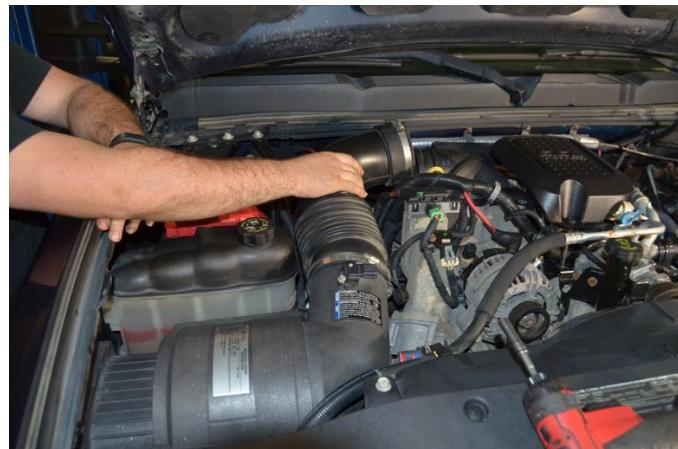
2. Remove the Resonator from the turbo mouthpiece.
