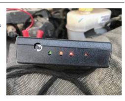
FLASH CODES: FLASH CODES ARE FLASHING LIGHTS ON EACH OF THE LED'S, THE NUMBER OF EACH ONE (RUNNING FROM LEFT TO RIGHT) WILL INDICATE THE ERROR EXPERIENCED.
